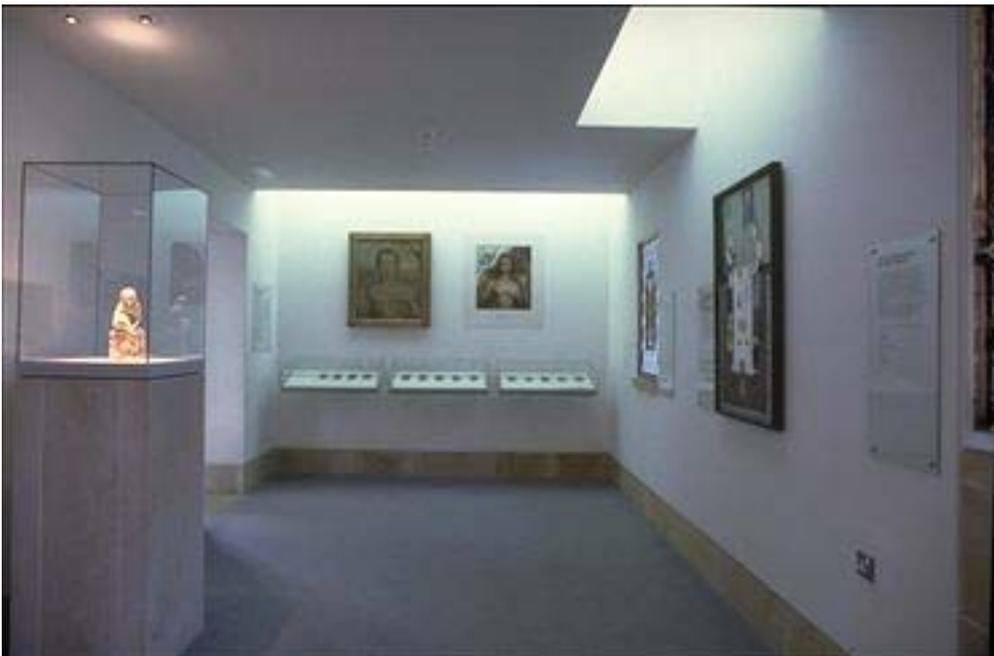
2 Low Light Gallery, St. Mungo's Museum. Low light levels are accomplished by creating coffers over display cases with Durer miniatures. Bouncing the light round the coffer and down the wall provides at once an even coverage at 50 lux without dimming and a uniform visual environment allowing high visual acuity without glare or problems of the viewer self shadowing the lightsource when closely examining the exhibits.
